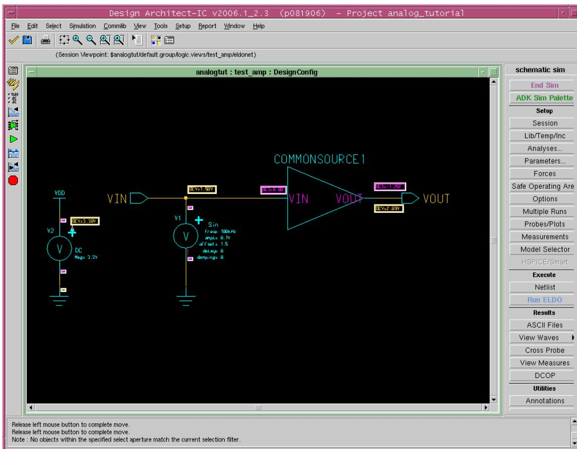
Current and Voltage values at various nodes will be displayed as shown in the above figure.
