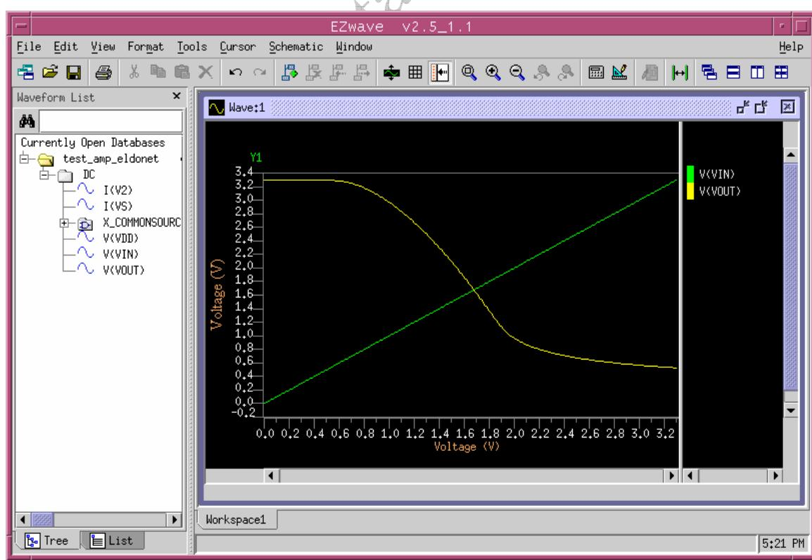
This DC analysis shows you where to set the DC bias point of the transistor. From the input/output plot, we see that the high gain region corresponds to a DC input voltage of about 1.0V to 1.8V. In the subsequent analyses, you will set a DC bias voltage of 1.5V at the gate of the transistor, ensuring that the device is operating in the the correct region.
